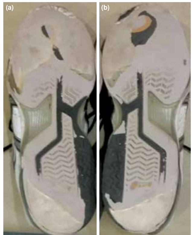
Figure 2. (a, b) Wear pattern on bottom of right and left tennis shoes. In left shoe with less total contact area and higher pressure values, there was more wear compared to right shoe.
