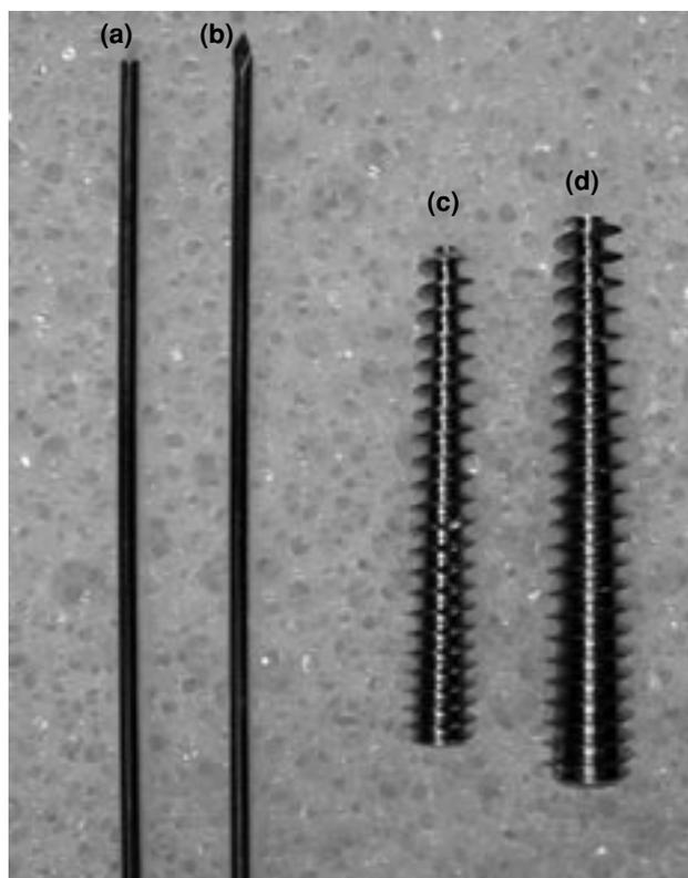
**Fig. 1.** (a) Flat and (b) sharp ends of the K-wire. (c) Mini-Acutrak screw, (d) standard Acutrak screw.
