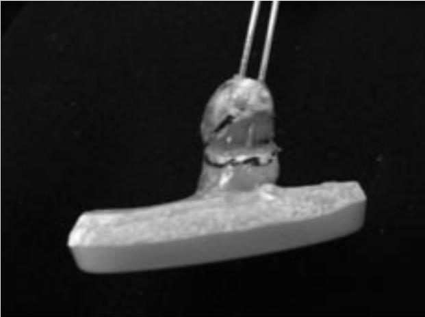
**Fig. 2.** Potted scaphoid model showing placement of parallel K-wires.
