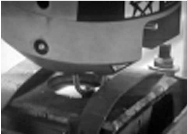
Figure 1. Pedicle screw was fastened to the upper jaw by a U-shaped apparel. The blue cube in the metal box is the Amberok model stone containing the embedded vertebra. The blue cube is secured in the metal box while the box helped to fasten to the lower jaw.
