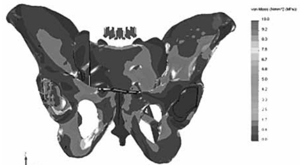
Figure 7. Tension distribution on the model: maximum value: 750 MP (deformation magnified 3x).
