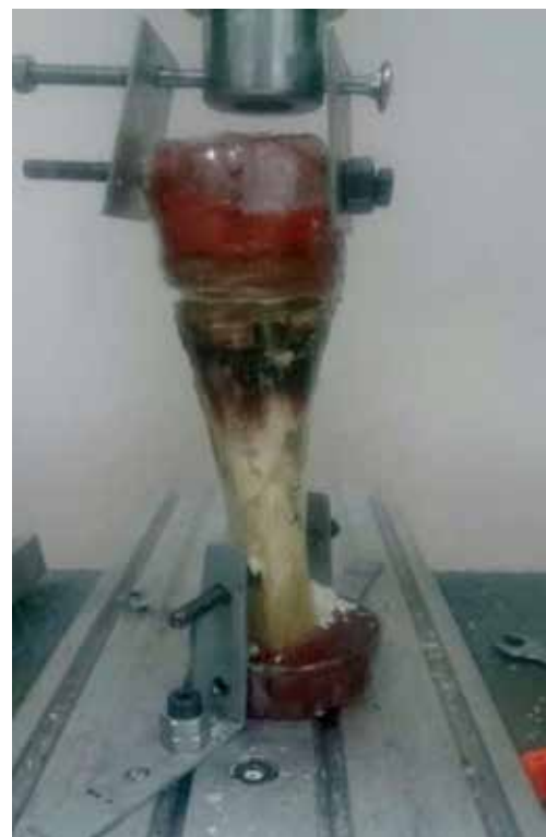
Figure 4. Bicortical screw tensile force application.
