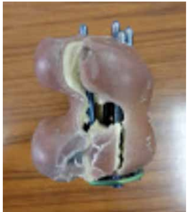
Figure 3. Failure appearance on axial plane after load to failure tests.
