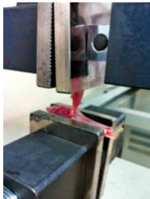
Figure 2. Muscle components with muscle tendon junction were attached to supernatant moving holder.
