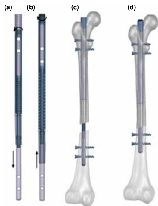
Figure 1. Schematic drawings of nailing mechanism. (a) The view of established system before application. (b) The view of the system activated during application. (c) Stage of the implantation of the system to the bone. (d) The view of the system which was activated after fixation.
