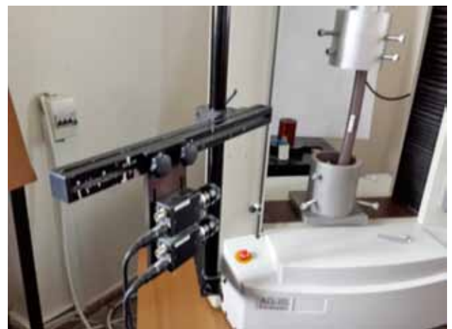
Figure 4. Video extensometer at left side and optic marker on composite femur in universal test machine.
