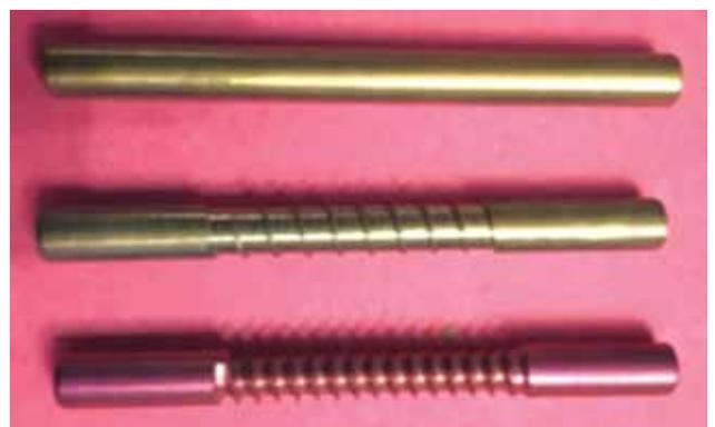
**Figure 1.** Unthreaded, low threaded, and high threaded titanium screws.
