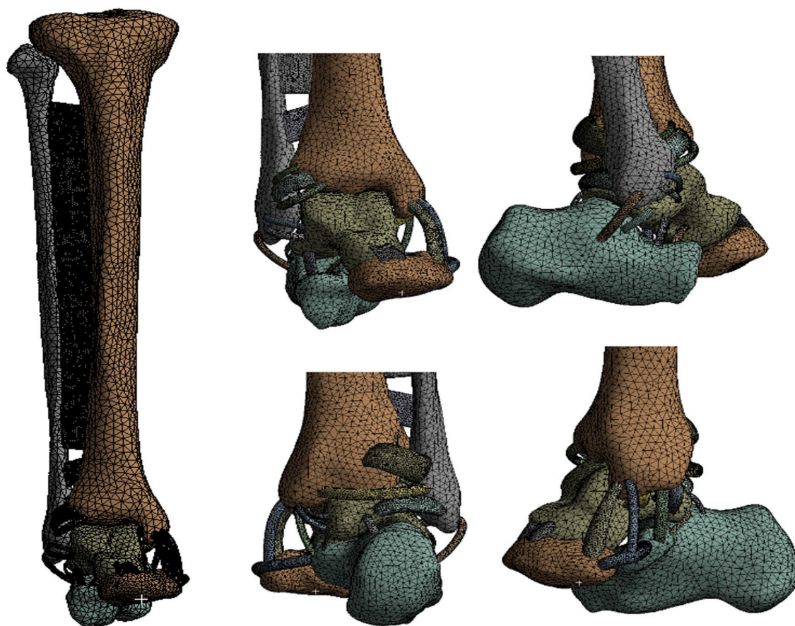
FIGURE 1. Lower extremity ligaments, interosseous membrane and finite element model mesh structure.
