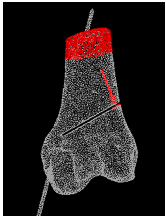
FIGURE 3. Loading and boundary conditions. Distal femur was fixed at the proximal end and load was applied perpendicularly at the osteotomy site.
