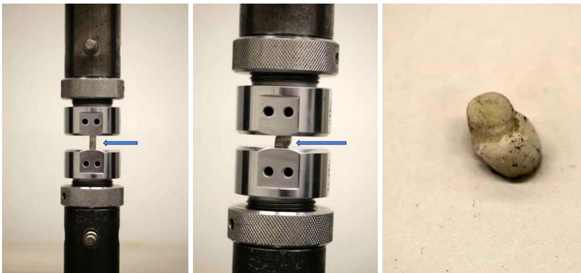
**FIGURE 3.** Compressive load test machine. A cement block (arrow) was secured between the two arms of the machine, which compressed the cement block at a rate of 25 mm/min. The maximum compressive load was automatically measured when the cement block was crushed.
