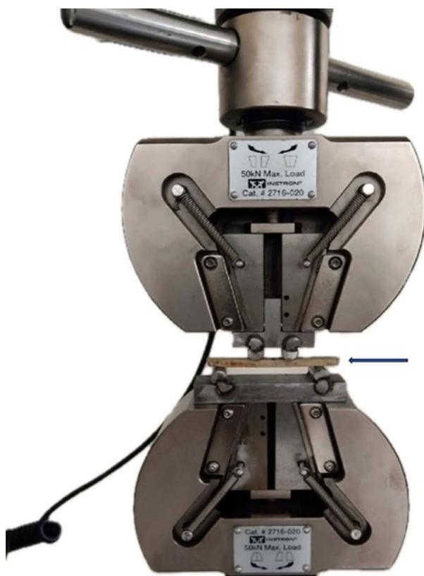
**FIGURE 2.** Four-point bending load test machine. A cement block (arrow) was sandwiched between the fixtures. The speed of the device was set to 5 mm/min. The maximum four-point bending load was automatically measured when the cement block was fractured.
