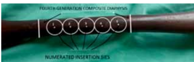
Figure 2. Numbered screw insertion sites on artificial femur diaphysis.
