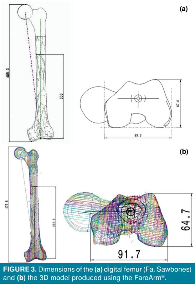
**FIGURE 3.** Dimensions of the (a) digital femur (Fa. Sawbones) and (b) the 3D model produced using the FaroArm®.
