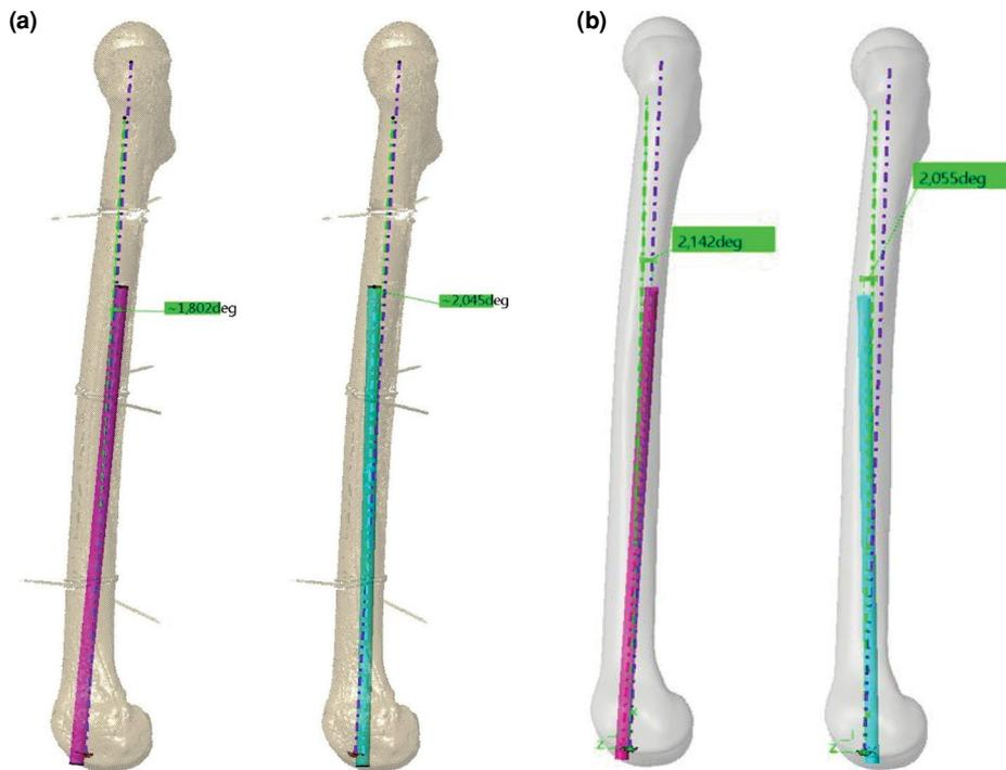
**FIGURE 8.** Maximal angulation errors for 5 mm anterior (purple) and 5 mm posterior (turquoise) displacement for (a) FaroFemur and (b) DigitalFemur in the sagittal plane.
