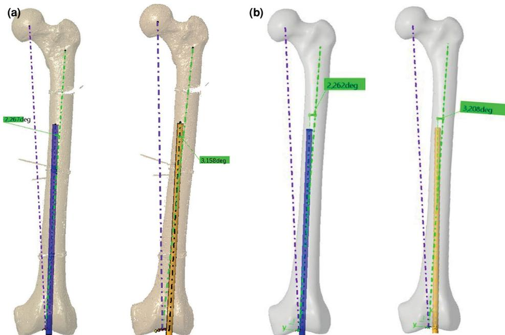
**FIGURE 7.** Maximal angulation errors for 5 mm (blue) and 10 mm (light orange) lateral displacement for (a) FaroFemur and (b) DigitalFemur in the coronal plane.
