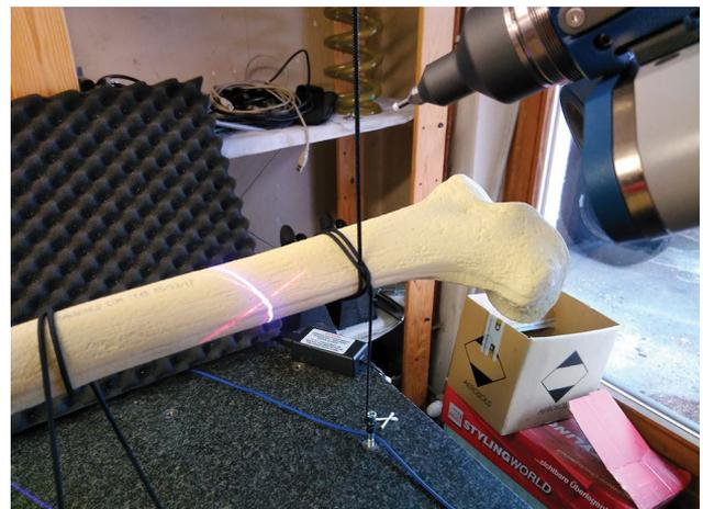
**FIGURE 2.** Scanning of the analogue large femur model using FaroArm®
