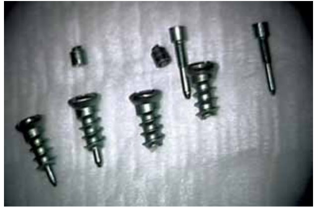
Figure 5. Broken osmium screws.
